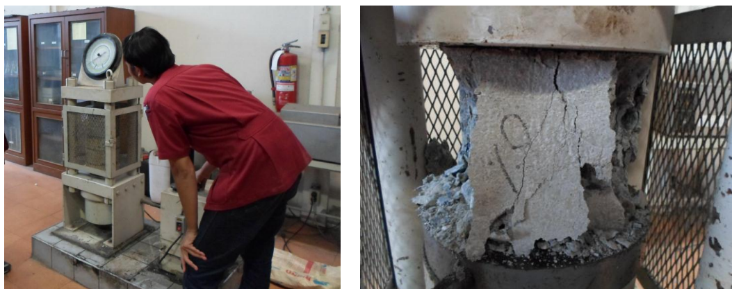
Figure 5. Cube specimen compressive strength test
