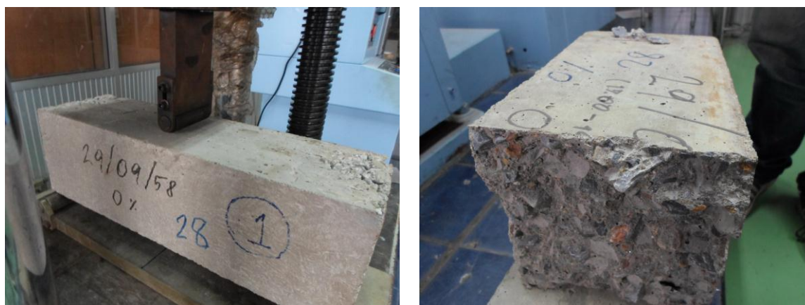
Figure 7. Beam specimen loading arrangement (flexural strength test)
